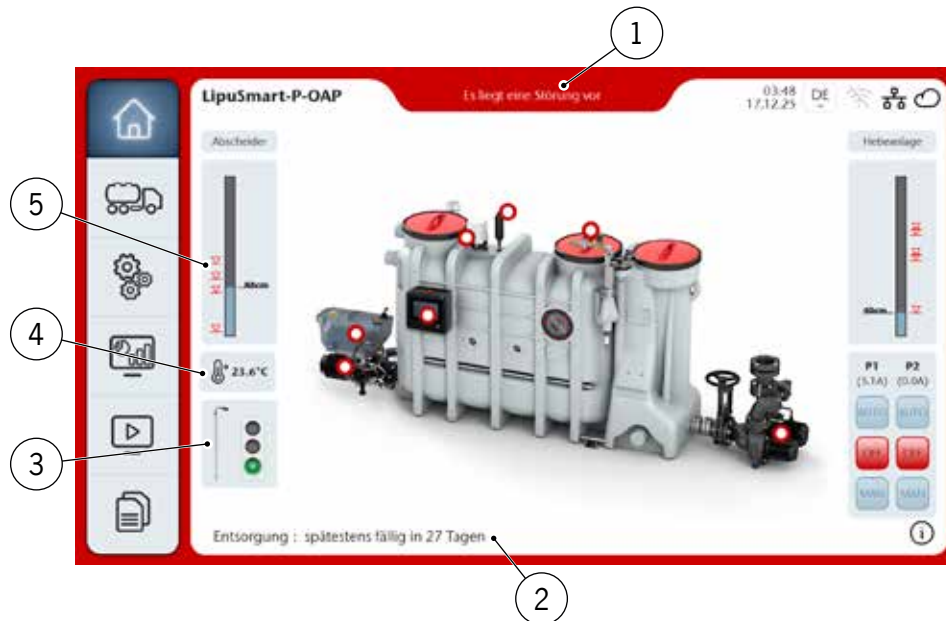
Figure: Status display of the grease separator
