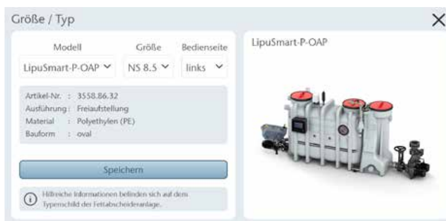
Figure: Selection of the installed grease separator system
